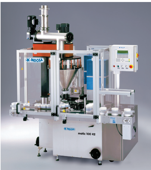
INDOSA matic 100 K2 with filling station INDOSA TR2 for filling and double-sealing of cardboard lids onto composite cans.
