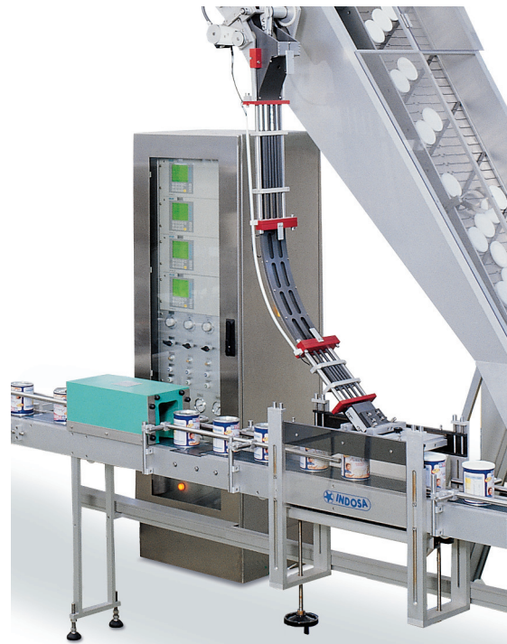
Control unit for gassing system „proGAS“, can transport system with can turning device and over-capping system
