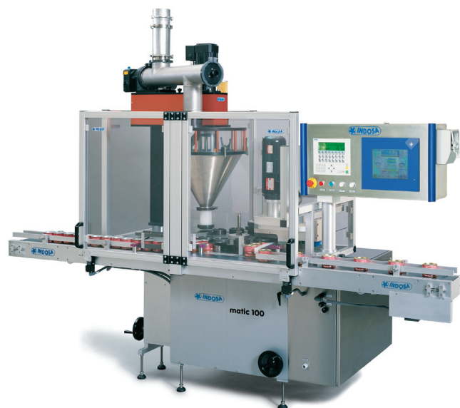
INDOSA matic 100-02 with filling station INDOSA TR2 for filling and seaming of tin lids onto tin cans or composite cans.
